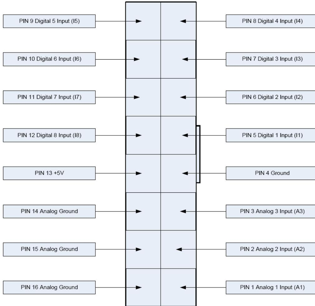
Figure 9.0 WebControl™ J12 Input pins
