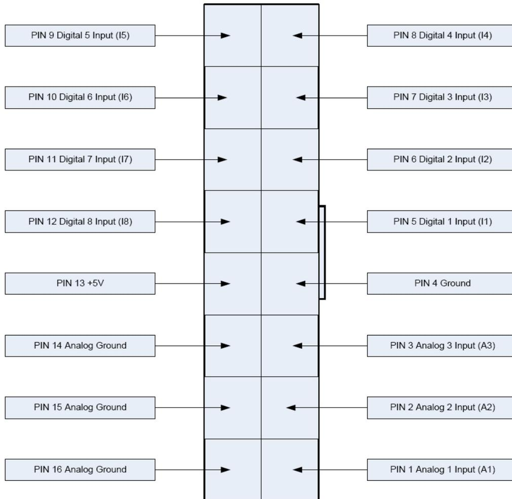
Figure 9.0 WebControl™ J12 Input pins
