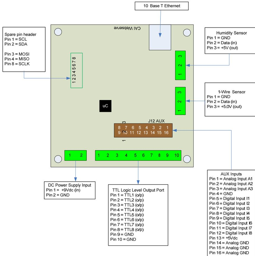
Figure 1.0 WebControl™ PCB inputs and outputs diagram
