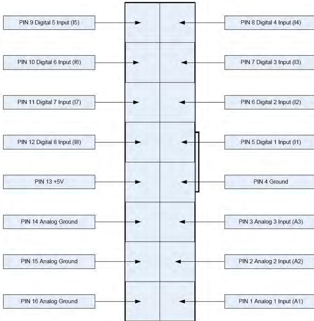
Figure 7.0 WebControl™ J12 AUX I/O Connector
