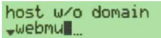
Enter the host name of the WebMux. Use the right arrow to move the position, the up and down arrows to select characters, left arrow to move back in position, check mark button to confirm the change. This host name is for identification purposes. You may call it webmux1, webmux2, etc. (You can hold down the up/down button for more than a second to make quicker changes.) Note the left most down arrow on the LCD allows the user to move to other settings.
