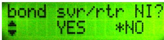
This option will allow you to use the “Internet/rtr” port and “Server/svr” port as a single “bonded” interface, also known as Port Channel or Link Aggregation Group, allowing substantially more data throughput than a single physical interface. Please refer to Appendix N for details.
