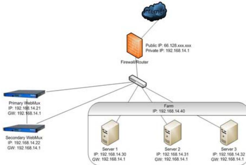
Single Network Mode configuration is simple, with only one interface connected to the network. You can use either the Internet Port or the Server Port of the WebMux, but only ONE of them. The WebMux and the servers are also all on the same subnet.
